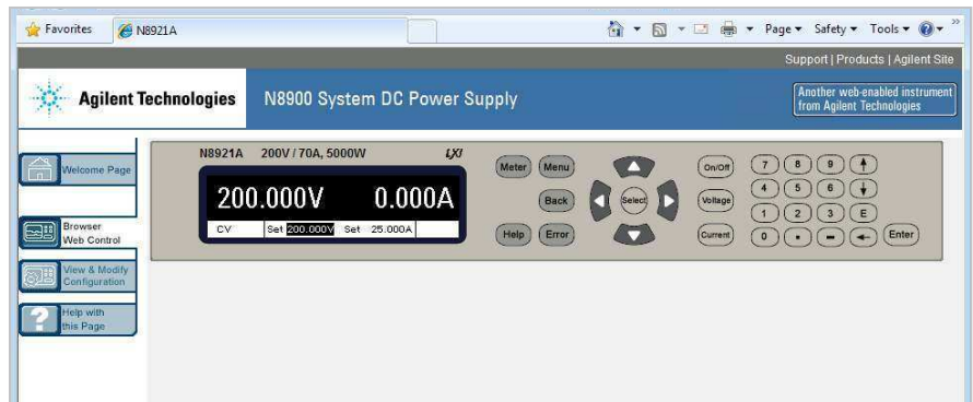
Figure 3. N8900 Series web graphical user interface for remote access and control of the power supply
