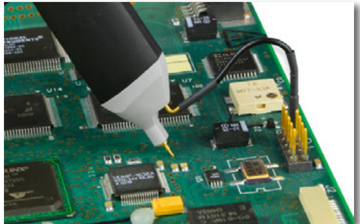
Use the spring-loaded Pogo Tip to maintain reliable contact with small probe points. Use this tip with any of the ground leads like the flexible Short Right-Angle Lead shown here.
