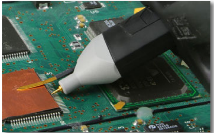
The Ground Blade and Copper Pad provide the shortest ground loop for excellent signal fidelity when probing an IC.
