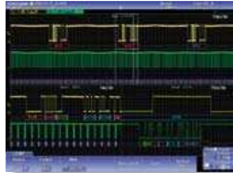
Simultaneous analyses of CAN and LIN
