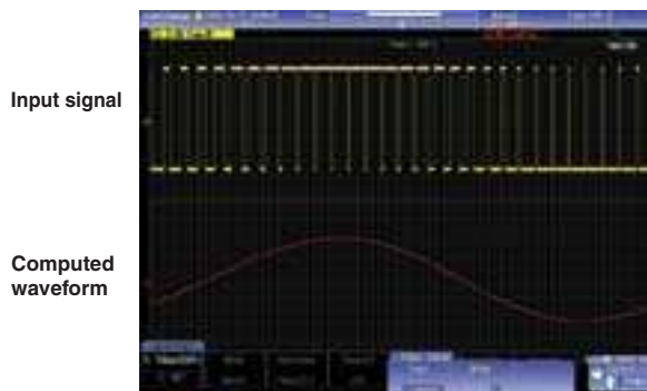
Filtering of a PWM waveform using computation
