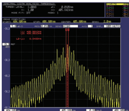
405 nm FP-LD measurement (resolution setting: 0.01 nm)
