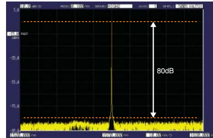
Example of the stray-light suppression ratio High dynamic mode: OFF, Resolution setting 0.1 nm, High performance model
