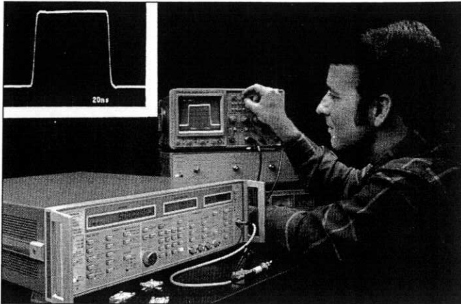
Built-in pulse generator typically has less than 5 ns rise time over a 25 ns to 99 ms pulse width range.
