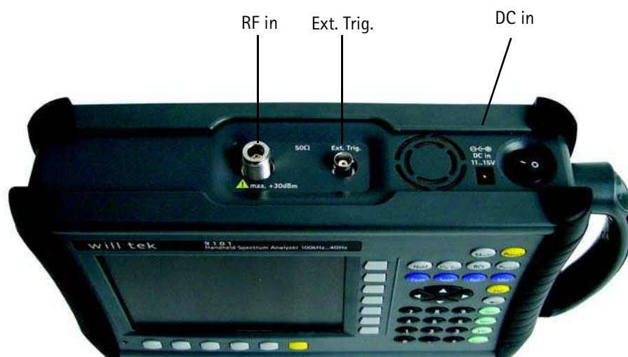
Figure 1 9101 connectors on the top of the instrument
