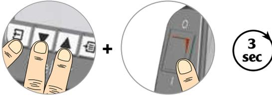
When switching on: Exit, UP and DOWN until a signal sounds
