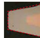
Weller WSW after 10,000 solder cycles
