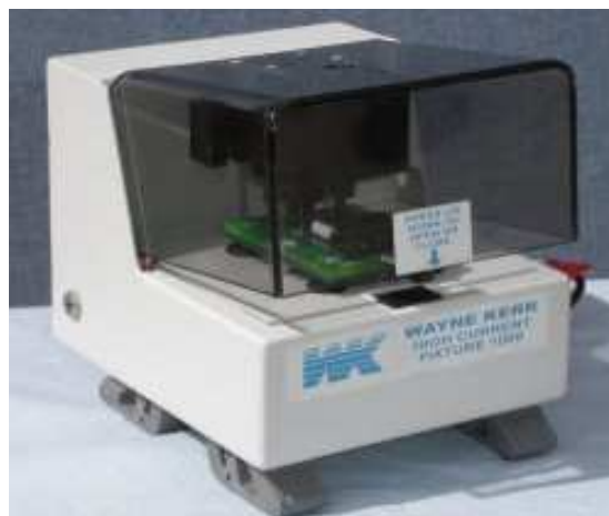
Figure 2-4 1009 High Current Fixture
