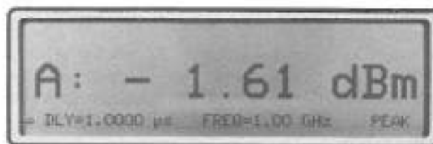
Figure 3-2. Typical Single Channel Peak Power Display
