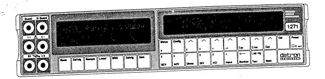
The two displays on the front panel deal with different aspects of operation. We set up the instrument's configuration using menus shown in the right-hand (dot-matrix) display, then readings appear in the left-hand (main) display.
