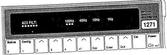
This menu permits any one of four integration filters to be used for the AC Current measurement. It defines the following *choice* keys, each selecting a filter with recommended lowest frequency as shown below and on the dot-matrix display:
