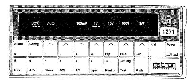
There are two classes of front panel menu keys; those that lead to an immediate change of instrument state (i.e the major function keys DCV, ACV, Ohms, DCI, ACI), and those that do not (Status, Config, Cal, Input, Monitor, Test, Math).
