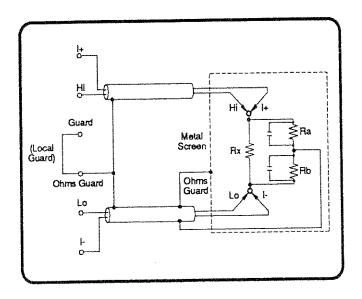
' $\Omega$  Guard' can be used to make 'in-circuit' resistance measurements by guarding out parallel resistance paths so that only the value of Rx will be displayed.
