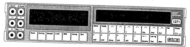
The two displays on the front panel deal with different aspects of operation. We set up the instrument's configuration using menus shown in the right-hand (dot-matrix) display, then readings appear in the left-hand (main) seven-segment display.
