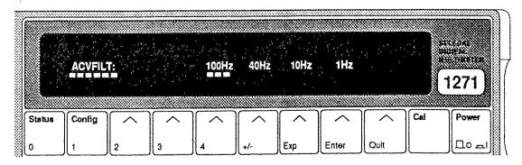
This menu permits any one of four LF filters to be used for AC Voltage measurement. Each *choice* key selects a filter whose lowest pass frequency is as shown.
