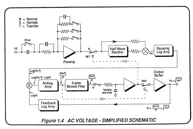
The Log Amp squares instantaneous values of its input by converting them into logarithmic values, then multiplying by two. Its instantaneous log output currents have a DC current proportional to logVf subtracted from them. The result is a current (proportional to log[Vin²] - logVf) which is fed to an 'exponential' stage.
