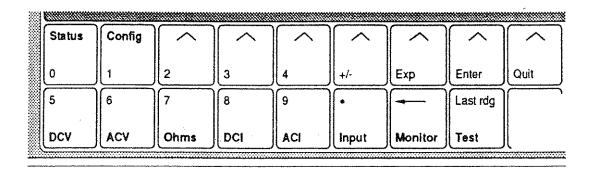
Some menu and soft function keys, shown above, also act as a keyboard for entry of parameters such as math constants, limits, bus address, etc. The data entered is purely numeric, and can consist of either a keyboard-entered value or the value of the most recent reading.
