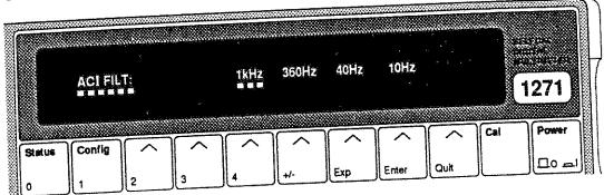
This menu permits any one of four integration filters to be used for the AC Current measurement. It defines the following *choice* keys, each selecting a filter with recommended lowest frequency as shown below and on the dot-matrix display:
