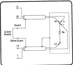
above about  $1M\Omega$ , a metal screen can be wrapped around the resistor to reduce noise. Connecting the  $\Omega$  Guard terminal to the screen will intercept leakage via the screen (in parallel with the unknown resistor). The resistor under test should not be grounded, as this will make the measurement noisier.
