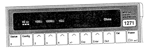
The HI $\Omega$  menu gives access to the three higher ranges not present on the normal OHMS menu. The 'Autorange', 'Fast' and 'Low Current' facilities are not available, and the range of resolutions is restricted. It defines the following keys:
