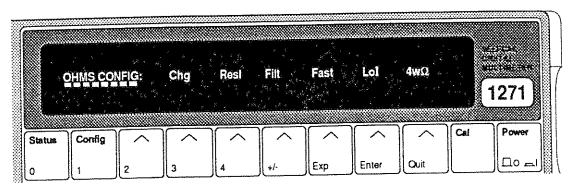
Chg and Resl are menu keys, but  $\underline{Filt}$ ,  $\underline{Fast}$ ,  $\underline{Lol}$ , and  $\underline{4w\Omega}$  are toggle keys.
