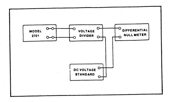
Figure 5-1. Test Equipment Connections.
