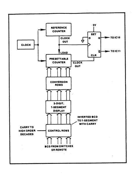
Figure 4-3. Block Diagram, Variable Reference Source.
