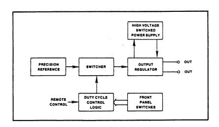
Figure 4-1. Block Diagram, Model 2701B Precision DC Voltage Calibrator.
