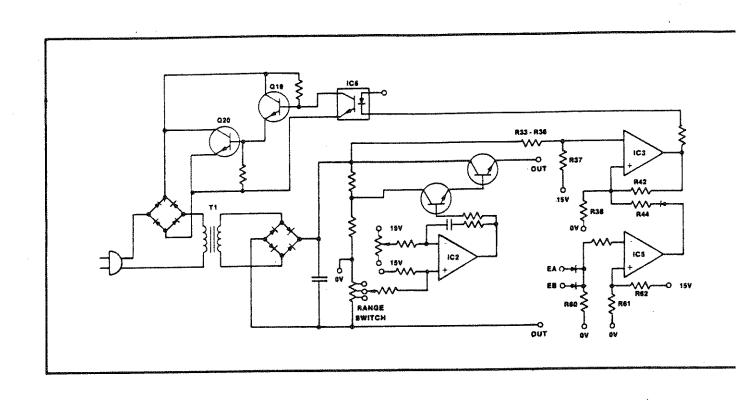
Figure 4-2. Simplified Schematic Diagram, Model 2701B Precision DC Voltage Calibrator.
