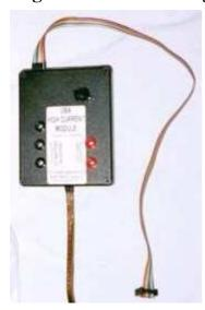
This module allows discharging a battery at up to 15 Amperes (or 50A with the Very High Current Discharge Module). It works in conjunction with a load that you supply and a UBA4. It connects and disconnects the load while measuring the load current. For the load, you can use automotive lamps, power resistors or even an active load.
