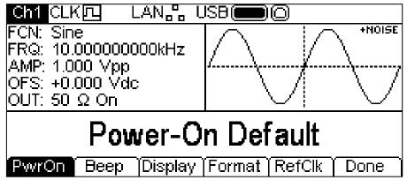
With **Power-On Default** selected the instrument will power up with the factory default parameters loaded.
