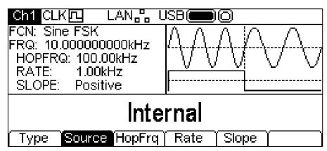
To select the modulation source press the **Source** soft-key. The options are **Internal** or **External**. Internal will use an internally generated trigger signal, external will use the signal present at the TRIG IN connector and the **Rate** soft-key will disappear. The Graph Box will show a switching carrier and a square-wave as the modulating waveform irrespective of the source of the switching signal.
