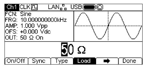
This is the value that is assumed to be loading at the instrument MAIN OUT connector. The value is used to calculate the actual values of amplitude and dc offset. Note that the output impedance of the instrument MAIN OUT connector is fixed at  $50\Omega$ .
