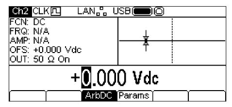
There are no **Freq** or **Amp1** soft-keys and the **Offset** soft-key has changed to **ArbDC**. The Parameters Box shows **DC** in the **FCN** field, the Graph Box shows a dc waveform with dc offset arrows and the Edit Box contains the dc voltage menu. The voltage may be changed in either of the ways detailed in General: Numeric Editing.
