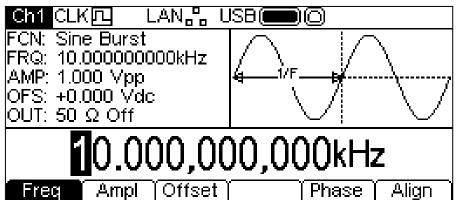
Notice that <code>Burst</code> still shows in the <code>FCN</code> field of the Parameters Box and the BURST key still glows yellow indicating that burst is still active. To return to the Burst menu to edit the burst parameters press the BURST key again. To turn off burst press the BURST key while the Burst menu is displayed.
