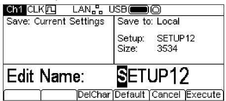
The name offered will be the same as the name in the selected set-up store when the **Save** soft-key was pressed. The Edit Box shows the name of the file that will be saved and the soft-key labels. KNOB and cursor keys allow the name to be edited.
