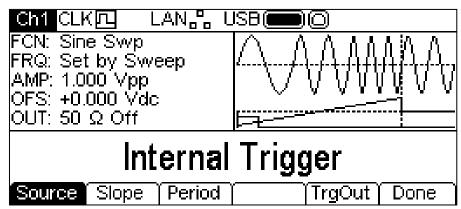
Repeated presses of the **Source** key will cycle round the four possible trigger sources:
