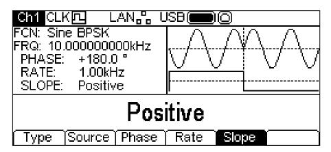
The options are **Positive** or **Negative**. Setting positive will cause BSPK to generate the BSPK Phase while the switching signal is high and the carrier phase while the switching signal is low. Setting negative will cause BPSK to generate the BPSK phase while the switching signal is low and the carrier phase while the switching signal is high.
