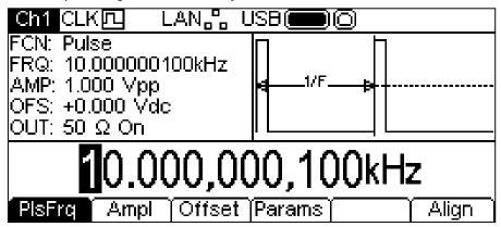
The PlsFrq soft-key allows setting of the pulse frequency. Pressing the key while it is highlighted will change it to PlsPrd and the pulse period may be entered. The pulse frequency may be changed in either of the ways detailed in General: Numeric Editing. The pulse generator uses its own value for pulse frequency/pulse period. Changing it will not affect the frequency/period value of the other carrier waveforms.
