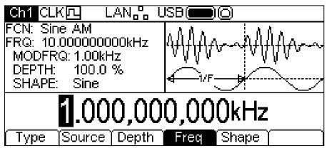
The frequency may be changed in either of the ways detailed in General: Numeric Editing. To set the modulation shape press the **Shape** soft-key. The currently selected shape will appear in the Edit Box and the soft-keys will change to a list of shapes available.
