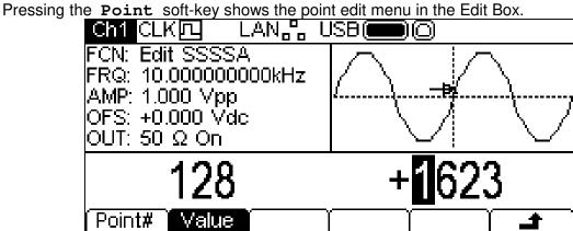
The point edit menu allows individual points in the waveform to be set to any vertical level value. The Point# soft-key selects setting of the point number; pressing the Value soft-key then enables the value to be changed. The point number and point value may be changed in either of the ways detailed in General: Numeric Editing. The point which is being edited is shown in the Graph Box by an arrow and a x. The point value is changed in the actual waveform immediately it is edited.
