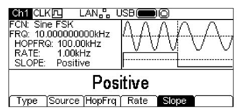
The options are **Positive** or **Negative**. Setting positive will cause FSK to generate the hop frequency while the switching signal is high and the carrier frequency while the switching signal is low. Setting negative will cause FSK to generate the hop frequency while the switching signal is low and the carrier frequency while the switching signal is high.
