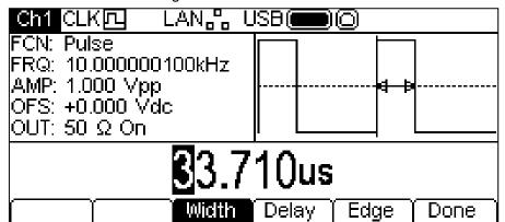
The Width may be changed in either of the ways detailed in General: Numeric Editing. Pressing the **Width** soft-key while it is highlighted will change it to **Duty** and the duty cycle may be changed in terms of the percentage of the pulse period.
