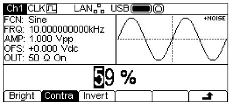
Pressing the **Bright** soft-key allows the display backlight brightness to be adjusted. The parameter may be changed in either of the ways detailed in General: Numeric Editing.
