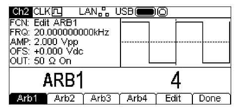
Note that the selected arb is available at the MAIN OUT connector of the selected channel during editing. This is shown by the **FCN** field in the Parameters Box showing **Edit NAME** where **NAME** is the name of the arb being edited. The original waveform will be output on exit from the edit menu.
