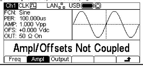
It is possible to set any combination of Frequency, Amplitude and Output coupling. When a parameter is coupled it may be changed on either channel and the other channel will also change.
