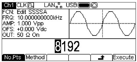
The No.Pts soft-key allows the new size to be specified. The number of points may be changed in either of the ways detailed in General: Numeric Editing. Press the Execute soft-key to resize the waveform and return to the top level edit menu. Pressing the soft-key will return without resizing.
