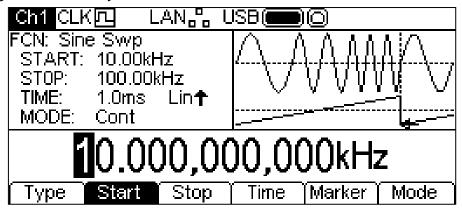
The Parameters Box now shows the current sweep parameters of **START** (frequency), **STOP** (frequency), **TIME** and **MODE** and **Swp** is shown in the **FCN** field. The **TIME** field also shows the sweep type. The Graph Box shows the sweep waveform type below a representation of the swept carrier waveform. The Edit Box contains the selected parameter, in this case start frequency.
