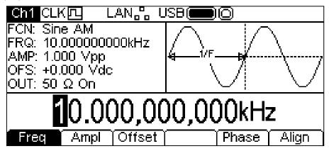
Notice that **AM** still shows in the **FCN** field of the Parameters Box and the MOD key still glows yellow indicating that modulation is still active. To return to the modulation menu to edit the modulation parameters press the MOD key again. To turn off modulation press the MOD key while the modulation menu is displayed.
