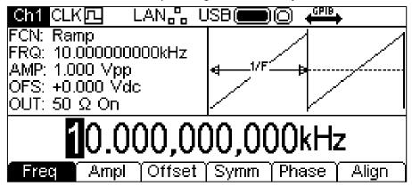
The RAMP key now glows green, the **FCN** field in the Parameters Box shows **Ramp** and the Graph Box has changed to show the ramp waveform.
