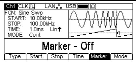
If the marker is disabled the Edit Box will show **Marker - Off**. To enable the marker press the **Marker** soft-key again.
