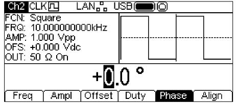
The phase may be changed in either of the ways detailed in General: Numeric Editing. The setting may be used to determine the phase difference between the the channels of a two channel instrument. The channels may be phase aligned by pressing the **Align** soft-key. The Phase parameter is also used to set Burst Phase and the phase between two generators. See the sections on burst and phase synchronising two generators for more details.
