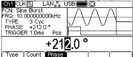
The phase may be changed in either of the ways detailed in General: Numeric Editing. The carrier waveform in the Graph Box will show a representation of the carrier start phase as the phase is edited. Note that the phase may also be set by pressing the **Phase** soft-key from the carrier menu.
