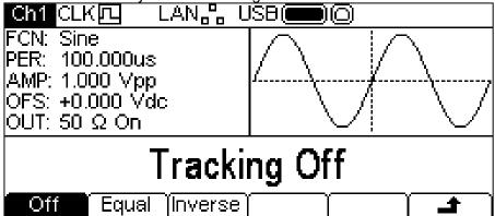
With Tracking Off the two channels behave independently and changes in parameters on one channel do not affect the other channel.
