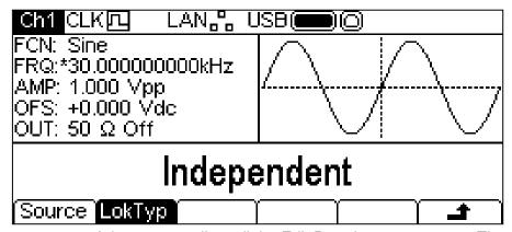
Press the **LocTyp** soft-key repeatedly until the Edit Box shows **Master**. The signal at the MAIN OUT from the generator will stop at the dc offset level.
