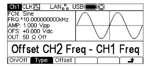
There are two types of frequency coupling available Offset CH2 Freq – CH1 Freq and Ratio CH2 Freq / CH1 Freq. Offset applies a fixed difference between the channels which is equal to Channel 2 frequency – Channel 1 frequency. Ratio sets the frequencies so that Ratio is equal to Channel 2 frequency divided by Channel 1 frequency.
