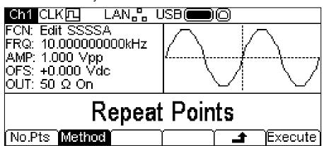
When a waveform is increased in size new points are added between existing points. The way that the values of these new points are calculated depends on the resize method setting, The **Repeat Points** method adds points of the same value as the original point in the waveform. The **Interpolate** method draws a straight line between the existing points.
