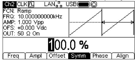
The symmetry may be changed in either of the ways detailed in General: Numeric Editing. To produce a triangle waveform set the symmetry to 50%.
