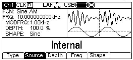
The Parameters Box now shows the current modulation parameters of MODFRQ, DEPTH and SHAPE and AM is shown in the FCN field. The Graph Box shows the modulating waveform below a representation of the modulated carrier waveform. The Edit Box contains the selected parameter, in this case modulation Source.
