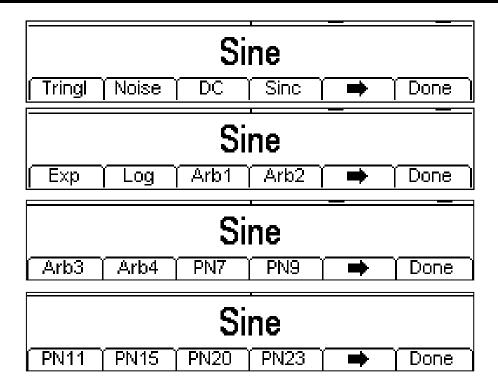
One more press of the soft-key will show the first list again. Select the modulation shape required by pressing the appropriate key then press the **Done** soft-key to return to the top level modulation menu.
