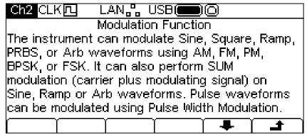
Below the topic heading is the topic text. If there is more text than will fit on the screen press the soft-key to scroll the text up one line. Continue scrolling until there is no more text indicated by the soft-key label disappearing. Once the text has been scrolled the soft-key may be used to scroll the text up one line. Pressing the soft key will return to the previous screen.
