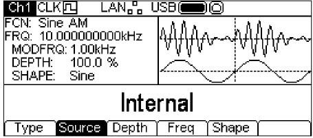
To select the modulation source press the **Source** soft-key. The options are **Internal** or **External**. Internal will use the waveform specified in the shape parameter and the Graph Box will show that shape as the modulating waveform. External will use the signal present at the MOD IN connector and the **Freq** and **Shape** soft-keys will disappear. The Graph Box will always show a sinewave as the modulating waveform if the source is set to External.
