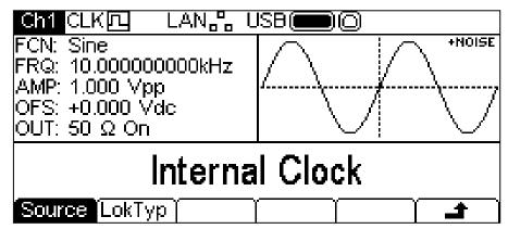
Pressing the Source soft-key will alternately select between Internal Clock or External Clock. With internal clock selected the instrument will use its internal TCXO as the timing reference for the creation of all waveforms. With external clock selected the signal present at
