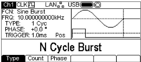
The Parameters Box now shows the current burst parameters of **TYPE**, **PHASE**, and **TRIGGER** and **Burst** is shown in the **FCN** field. The Graph Box shows the burst waveform trigger below a representation of the carrier waveform. The Edit Box contains the selected parameter, in this case type.
