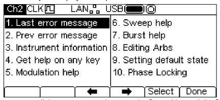
The Help menu uses all the screen space between the Status Line and the Soft-key Labels and contains a list of help topics. To show a topic use the  $\leftarrow$  and  $\rightarrow$  soft-keys to move the highlight back or forward through the list to select the required topic, then press the **Select** soft-key to show the topic screen.
