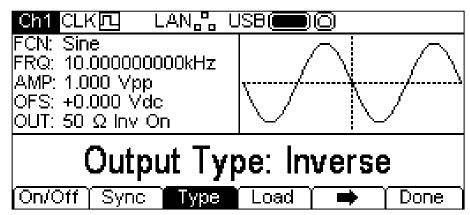
**Inverse** will invert the carrier waveform at the MAIN OUT connector. This is shown by **Inv** in the **OUT** field of the Parameters Box and the carrier waveform in the Graph Box will be inverted. Inversion is also possible using the +/- key as described in the Continuous Carrier Waveform Operation section.
