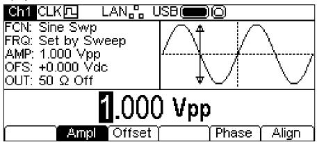
Notice that **Swp** still shows in the **FCN** field of the Parameters Box and the SWEEP key still glows yellow indicating that sweep is still active. To return to the Sweep menu to edit the sweep parameters press the SWEEP key again. To turn off sweep press the SWEEP key while the Sweep menu is displayed.
