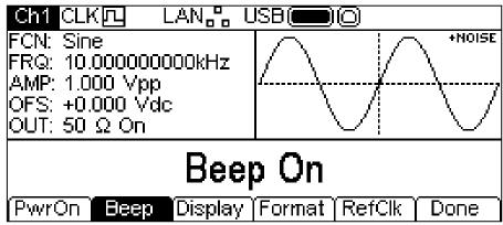
Pressing the **Beep** soft-key will alternate between **Beep ON** and **Beep Off**. With beep on the error and warning messages will be accompanied by a sound. These sounds are suppressed with beep off.
