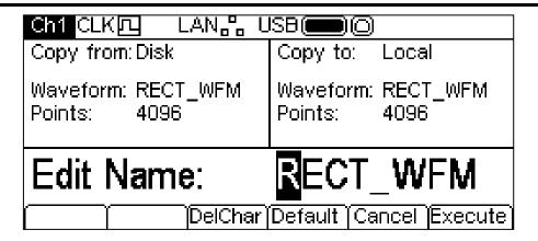
The Copy from: Box shows that the source is Disk and shows the file to be copied. The Copy to: Box shows the file that will be written to the local store. The Edit Box shows the name of the file that will be written and the soft-key labels. KNOB and cursor keys allow the name to be edited.
