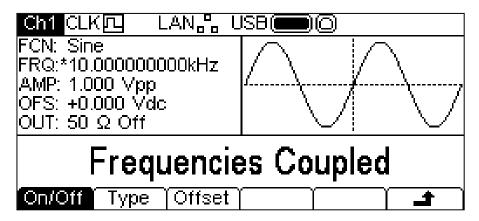
Use the On/Off soft-key to enable of disable frequency coupling. Note that \* is shown next to FRQ in the Parameters box.to indicate that the parameters are coupled
