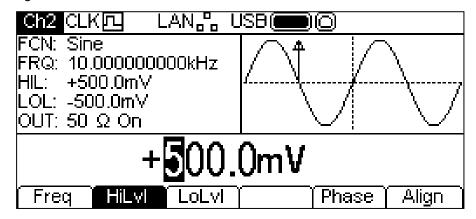
The selected parameter may be changed in either of the ways detailed in General: Numeric Editing. During a new entry the +/- key can be used at any time to set the value negative; alternate presses toggle the sign between + and -.
