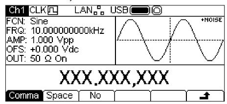
This menu allows the number format used in the Edit Box to be customised. The default is comma format which is selected by pressing the **Comma** soft-key. In comma format, digits after the decimal point are arranged in groups of three with the groups separated by a comma. Pressing the **Space** soft-key will change to space format.
