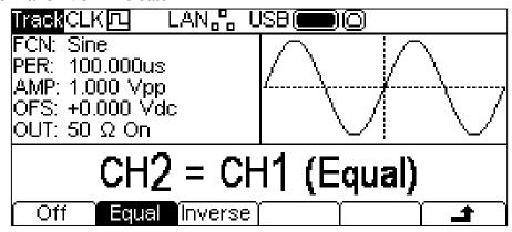
The channels can be set to track exactly by pressing the **Equal** soft-key, or Channel 2 may be inverted by pressing the **Inverse** soft-key to produce a differential pair of signals.
