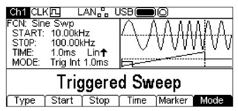
Pressing the **Mode** soft-key again while it is highlighted will return to continuous mode. All the parameters for sweep are now set.
