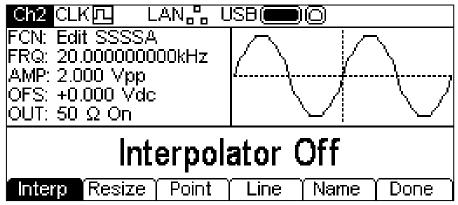
While editing an arbitrary waveform it will be available at the MAIN OUT connector of the selected channel for display on an oscilloscope. There is also a representation shown in the Graph Box and the **FCN** field in the Parameters Box shows **Edit Arbname** as a reminder that this waveform is temporarily selected for output.
