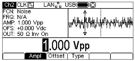
There is no **Freq** soft-key because the noise frequency cannot be edited. The amplitude or dc offset may be changed in either of the ways detailed in General: Numeric Editing. It is also possible to edit these parameters in terms of high level and low level.
