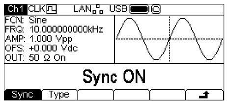
Pressing the **Sync** soft-key alternately turns the Sync Output off and on. To set the Sync type press the **Type** soft-key. The currently selected type will appear in the Edit Box and the soft-keys will change to a list of Sync types available.
