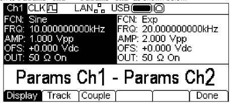
Here the Parameters boxes for both channels are presented together on the screen. The Parameters box of the selected channel is highlighted.
