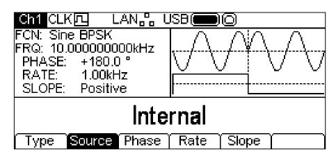
To select the modulation source press the **Source** soft-key. Internal will use an internally generated trigger signal, external will use the signal present at the TRIG IN connector and the **Rate** soft-key will disappear. The Graph Box will show a switching carrier and a square-wave as the modulating waveform irrespective of the source of the switching signal.
