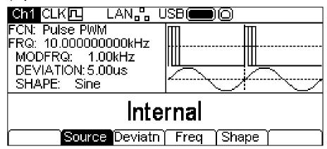
Note that PWM is the only modulation type applicable to pulse so there is no **Type** soft-key to allow selection of any other type.
