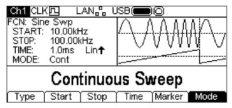
The default mode is Continuous Sweep. In this mode the sweep will proceed to the end and immediately start again with no pause. This is shown in the Graph Box by the sweep type waveform restarting immediately.
