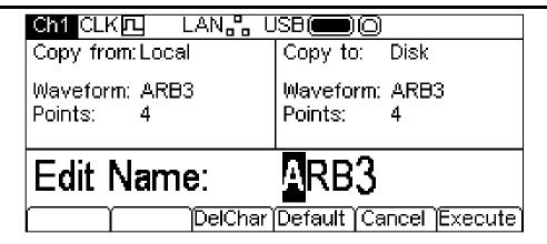
The Copy from: Box shows that the source is Local and shows the file to be copied. The Copy to: Box shows the file that will be written to disk. The Edit Box shows the name of the file that will be written and the soft-key labels. KNOB and cursor keys allow the name to be edited.
