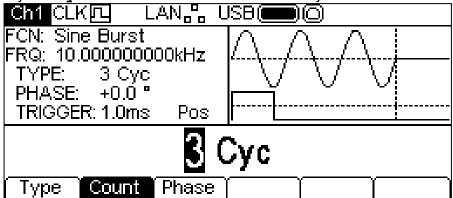
The count may be changed in either of the ways detailed in Numeric Editing Principles. The carrier waveform in the Graph Box will show a representation of the burst as the count is edited.
