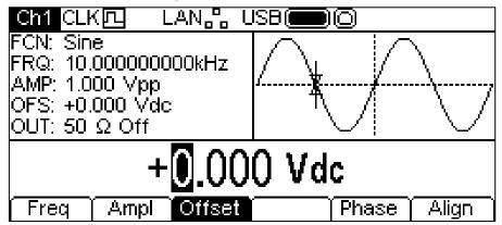
The offset may be changed in either of the ways detailed in General: Numeric Editing. During a new offset entry the  $\pm$ - key can be used at any time to set a negative offset; alternate presses toggle the sign between  $\pm$  and  $\pm$ .
