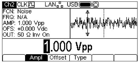
Pressing the Type soft-key shows the following and allows the PRBS function to be selected.
