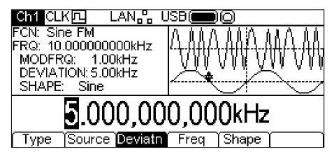
The deviation may be changed in either of the ways detailed in General: Numeric Editing. To set the modulation frequency press the **Freq** soft-key. The frequency parameter will appear in the Edit Box and the modulating waveform in the Graph Box will show that frequency is being edited.
