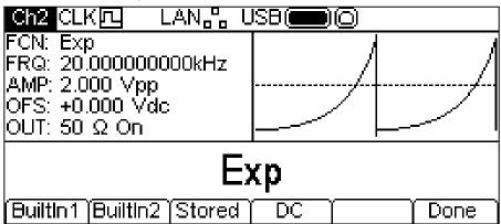
The soft-keys allow access to all the arbitrary waveforms in the instrument. **BuiltIn1** and **BuiltIn2** allow access to seven fixed waveforms which are built into the instrument and may be used like any other arb but cannot be edited. The **Stored** soft-key allows access to four waveforms which are user-defined and may be edited or loaded via any interface.
