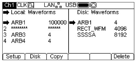
There are two operations available for waveform files as shown by the soft-key labels **Copy** and **Delete**. The copy operation will not be available if no USB flash drive is attached.
