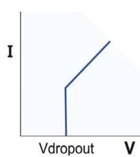
Resistive discharge (conductance mode) with voltage dropout.
