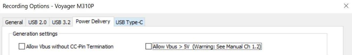
**Note** – *Allow VBUS > 5v* is a safety feature which prevents sourcing above 5V. When enabled, this mode will allow Voltage levels to be delivered to the DUT which may exceed their current carrying capabilities. While the Voyager system is designed to tolerate
