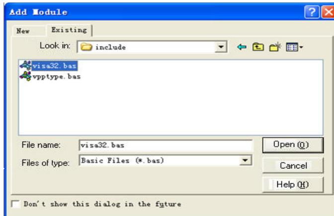
This allows the VISA functions and VISA data types to be used in a program.
