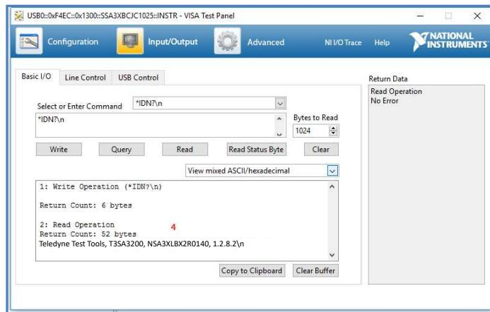
**NOTE:** The \*IDN? command (known as the Identification Query) returns the instrument manufacturer, instrument model, serial number, and other identification information.
