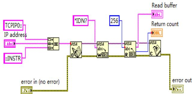
8、Input the IP address and run the program.
