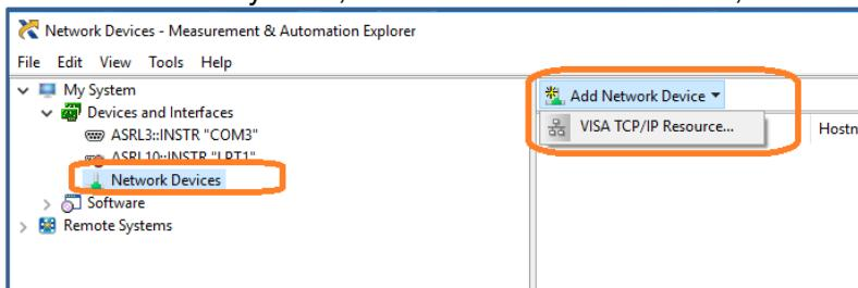
3. Select Manual Entry of LAN instrument, select Next, and enter the IP address as shown.
