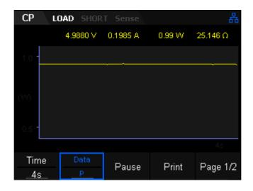
Figure 2-13 Waveform display interface of CP Mode
