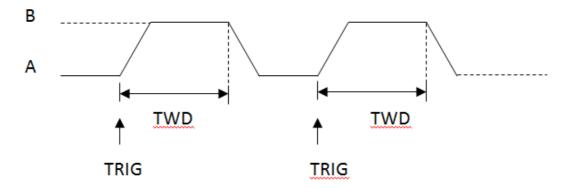
Figure 2-19 Transient CC Pulse Mode(Cont)
