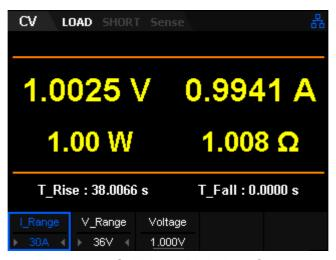
Figure 2-6 CV Mode Main Interface
