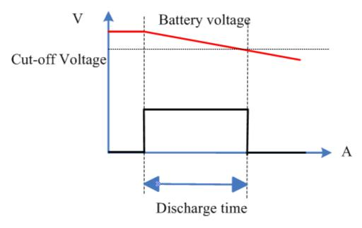
Figure 2-37 OPPT Test Function
