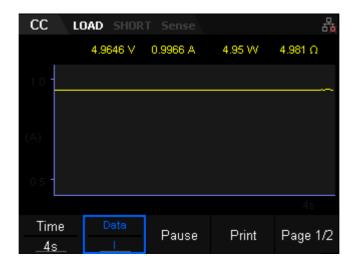
Figure 2-48 The waveform display in CC mode
