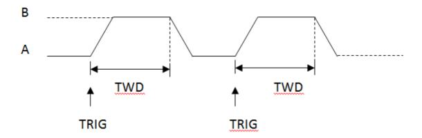
Figure 2-23 Transient CC Toggle Mode(Tog)
