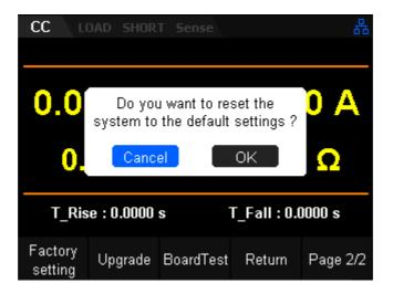
Figure 3-10 Restore factory setting interface
