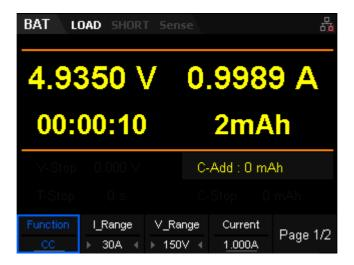
Figure 2-38 Battery Test Function
