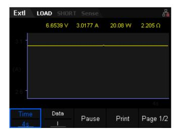
Figure 3-13 Waveform display interface of Extl mode
