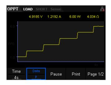
Figure 2-36 Waveform display interface of OPPT
