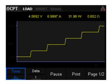
Figure 2-31 Waveform display interface of OCPT
