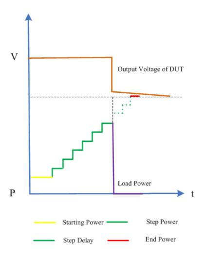
Figure 2-32 OPPT Test Function
