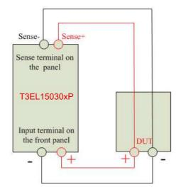
Figure 2-52 Sense connections
