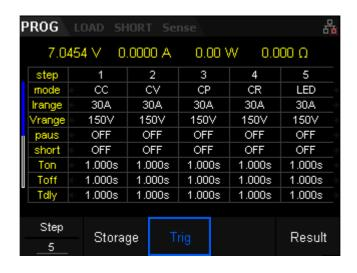
Figure 2-45 Program Test Function
