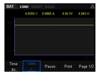
Figure 2-40 Waveform display interface of BAT
