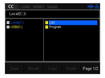
Figure 2-49 Storage and Recall Interface under CC mode
