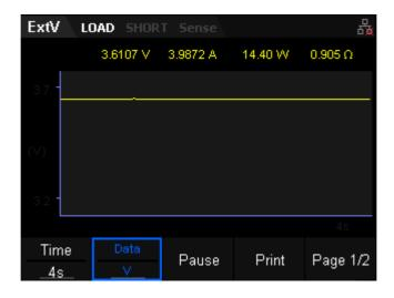
Figure 3-15 Waveform display interface of ExtV mode
