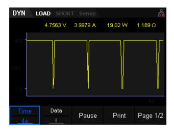
Figure 2-18 Waveform display interface of Cont mode
