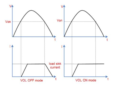
Figure 3-11 V - I characteristic curve of Von Latch
