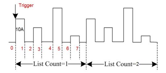
Figure 2-41 List Test Function
