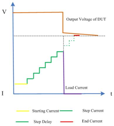
Figure 2-27 OCPT Test Function
