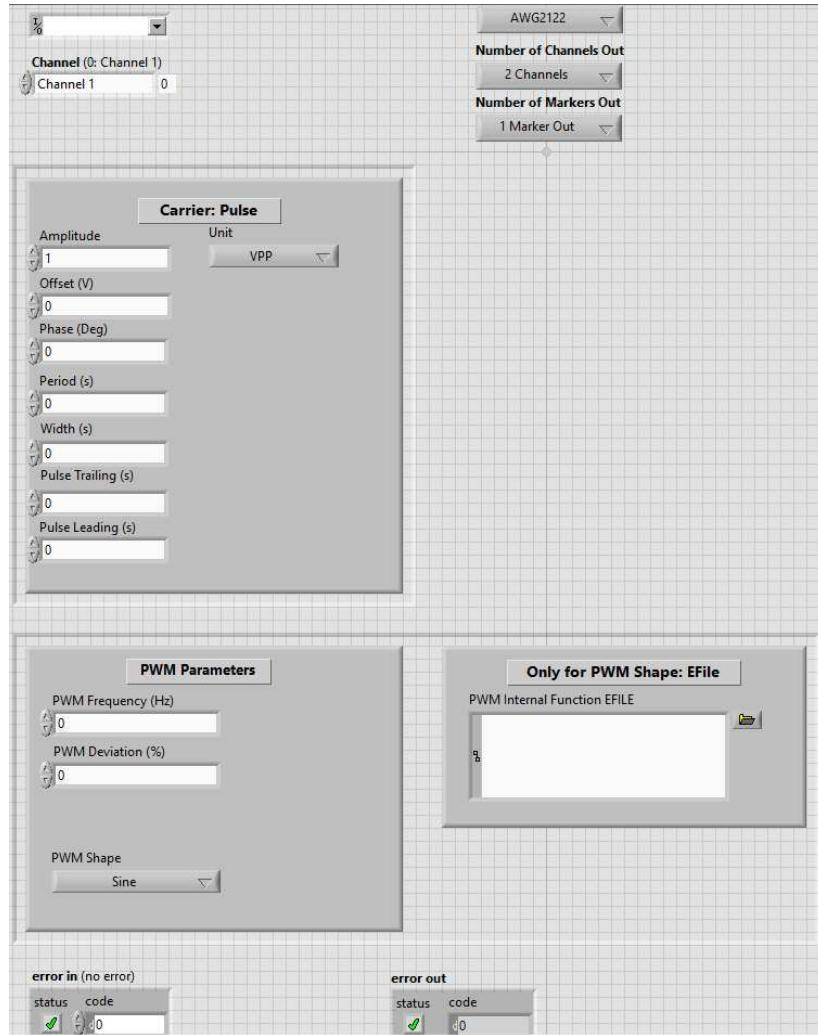
The PWM modulation is the only modulation supported by the Pulse waveform, so the carrier waveform is set Pulse by default.
