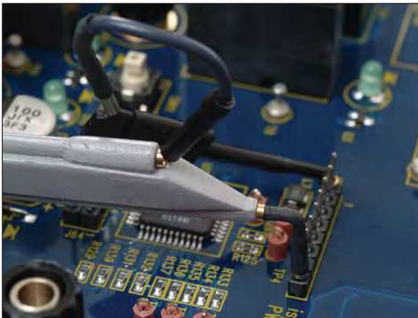
Use the Right-angle Connector and the Sprung Hook to probe square pins spaced far apart from each other.
