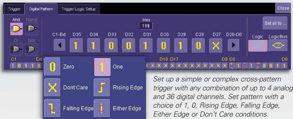
Use the oscilloscope triggers with digital channels.
