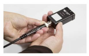
3. Slide up the sleeve so that it is flush to the body of the CA10 and completely covers the connector. Apply heat until the wrap snugly encases the connection.
