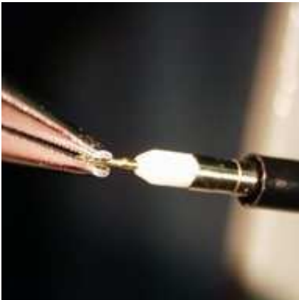
To remove a tip, grip the outmost portion and pull straight out.
