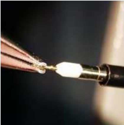
To remove tips, grip the outermost portion and pull straight out.
