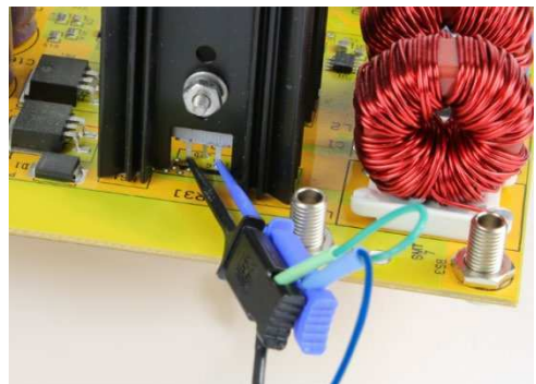
Properly connected tip when using stubs (left) or micro-grippers (right)
