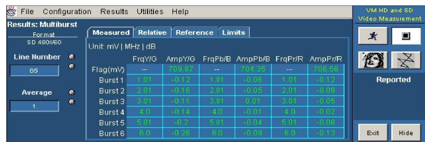
Figure 3-39: Displaying the Multiburst measurement
