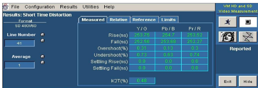
Figure 3-47: Displaying the Short Time Distortion measurement
