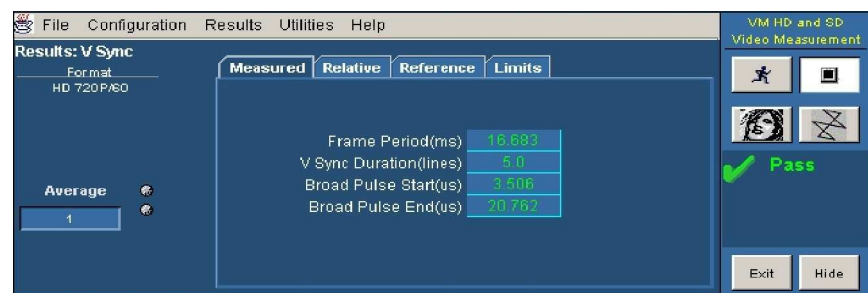
Figure 3-54: Displaying the V Sync measurement for HD Progressive format
