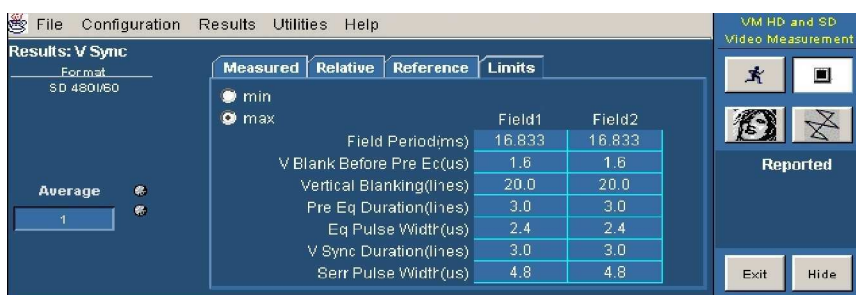
Figure 3-55: Displaying limit values for the V Sync measurement for SD Interlaced format
