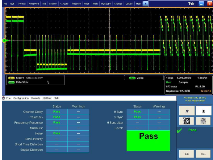
Summary Pass/Fail Test Results Display.
