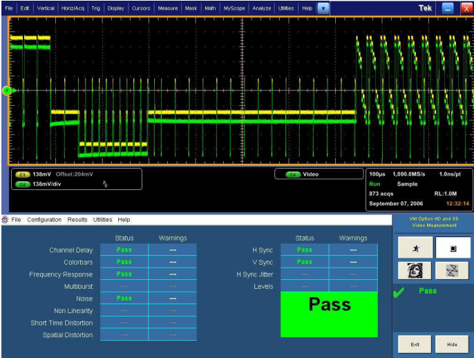
Summary Test Results Display with Pass/Fail Indication.
