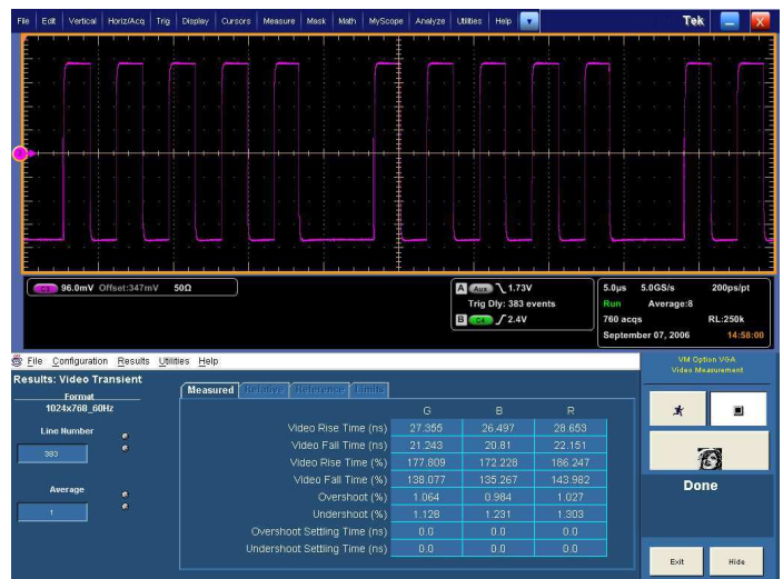
RGB Transient Response Measurement Results (Option VGA).
