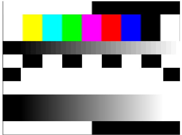
PC Graphics Matrix Test Signal (Option VGA).
