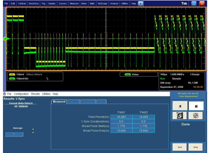
V Sync Display (Option SD and HD).
