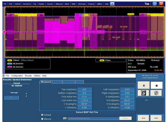
Spatial Distortion Display (Option SD and HD).
