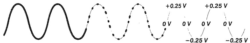
Figure 2-2: Acquisition: Input Analog Signal, Sample, and Digitize
