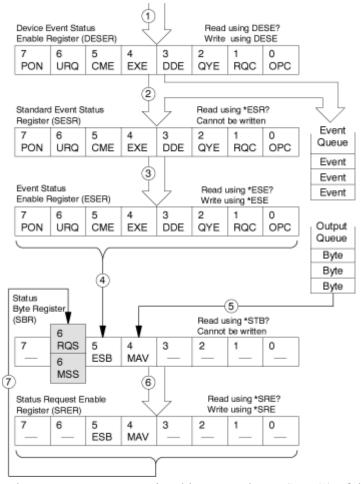
When an event occurs, a signal is sent to the DESER (1). If that type of event is enabled in the DESER (that is, if the bit for that event type is set to 1), the appropriate bit in the SESR is set to one, and the event is recorded in the Event Queue (2). If the corresponding bit in the ESER is also enabled (3), then the ESB bit in the SBR is set to one (4).
