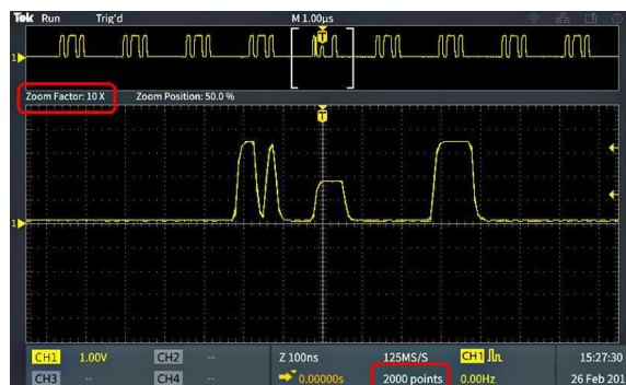
Maximum Zoomed waveform record captured with 2000 points
