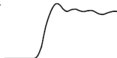
Signal with a long ground lead
