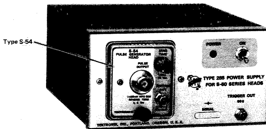
(C) Installed in Type 285 Power Supply Compartment
