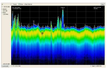
Swept DPX can capture low-probability events across spans greater than the real time bandwidth. Here, a 1 GHz sweep views the activity form 1.9 GHz to 2.9 GHz from an offair antenna. Number signals in the 1.9 GHz cell band are seen, and significant activity in the 2.4 GHz ISM band is apparent. The density measurement both has been used on the largest signal near the center, displaying approximately 3.5% occupancy.
