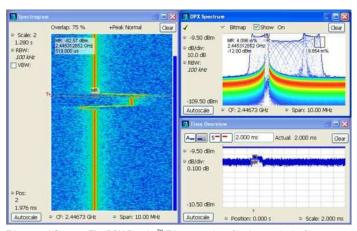
Trigger and Capture: The DPX Density<sup>™</sup> Trigger monitors for changes in the frequency domain, and captures any violations into memory. The spectrogram display (left panel) shows frequency and amplitude changing over time. By selecting the point in time in the spectrogram where the spectrum violation triggered the DPX Density™ Trigger, the frequency domain view (right panel) automatically updates to show the detailed spectrum view at that precise moment in time.
