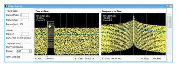
Pulse-Ogram displays a waterfall of multiple segmented captures, with correlated amplitude vs time and spectrum of each pulse. Can be used with an external trigger to show target range and speed
