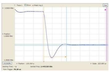
Settling time measurements (Opt. 12) are easy and automated. The user can select measurement bandwidth, tolerance bands, reference frequency (auto or manual), and establish up to 3 tolerance bands vs. time for Pass/Fail testing. Settling time may be referenced to external or internal trigger, and from the last settled frequency or phase. In the illustration, frequency settling time for a hopped oscillator is measured from an external trigger point from the device under test.
