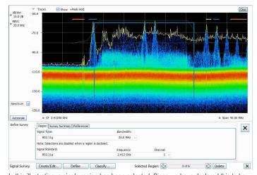
In this illustration, a single region has been selected. Since we have declared this to be an 802.11g signal, the spectrum mask for the 802.11g signal is shown overlaid in the region. The signal is a close match to the spectrum mask, However we can see some interferences with some likely Bluetooth signals in the ISM band
