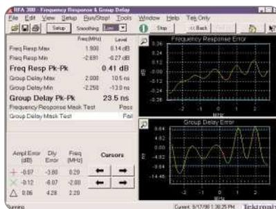
▶ *Frequency Response and Group Delay Measurements with Graphical Displays of Errors.*
