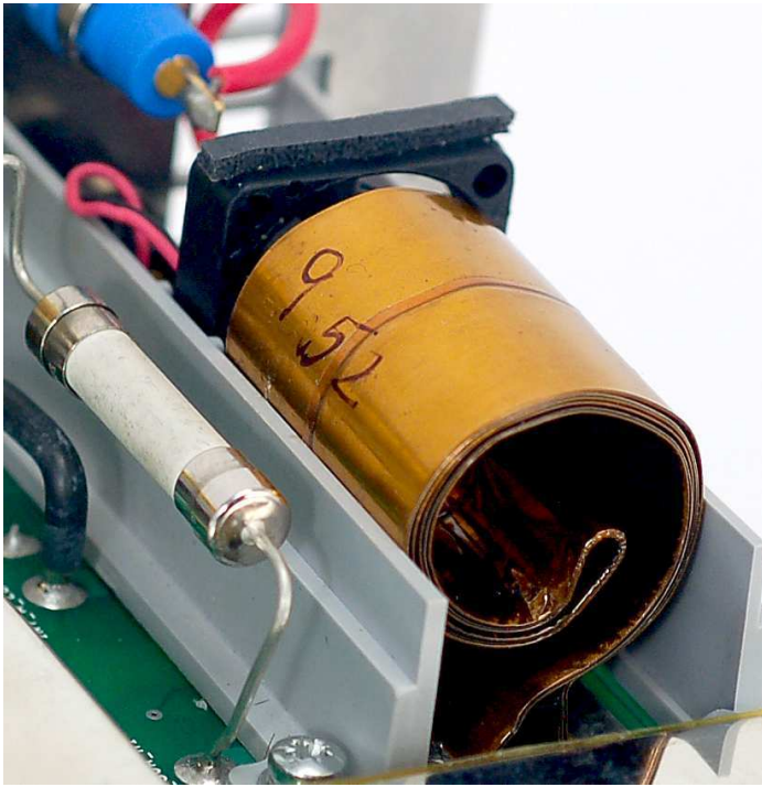
Spiral Shunt for 30 A input
