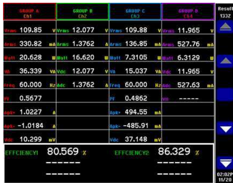
Figure 39: Efficiency measurement on the PA3000
