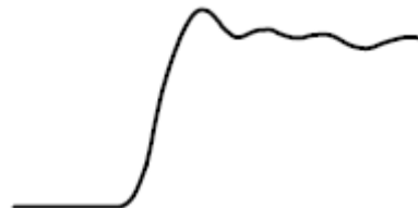
Figure 7: Signal with a long ground lead
