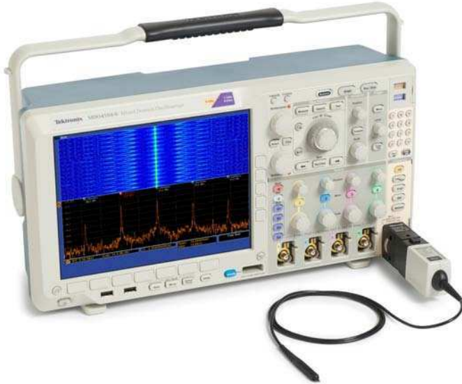
The optional TPA-N-VPI adapter enables any active, 50 \Omega TekVPI probe to be connected to the RF input.
