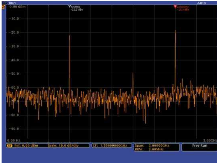
Spectral display of a bursted communication both into a device through Zigbee at 900 MHz and out of the device through Bluetooth at 2.4 GHz, captured with a single acquisition.
