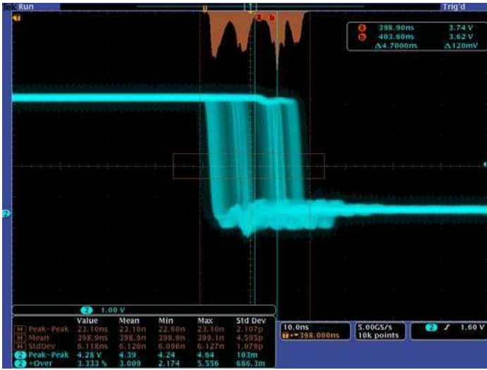
Analyze – Waveform histogram of a falling edge showing the distribution of edge position (jitter) over time. Included are numeric measurements made on the waveform histogram data. A comprehensive set of integrated analysis tools speeds verification of your design's performance.
