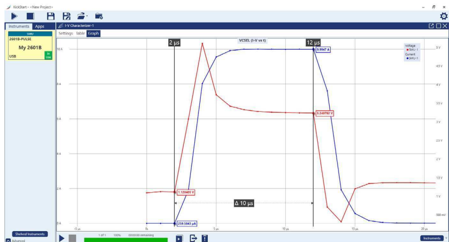
VCSEL Screenshot I-V-T for pulsing capability added as part of Slingshot project on the 2601B-Pulse SMU.
