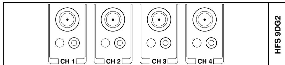
Figure 2-5: Channel Controls on an HFS 9DG2 Card
