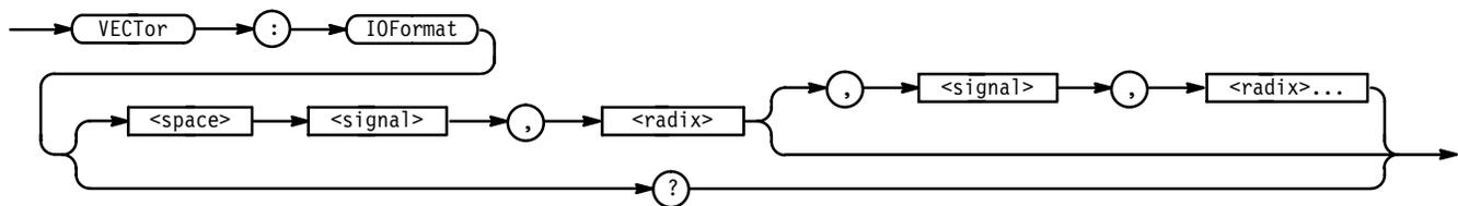
**Arguments** <signal> identifies the signal(s) to receive the data provided by subsequent BDATA commands.
