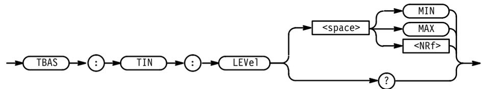
**Arguments** MIN sets the Trigger In level to the minimum.
