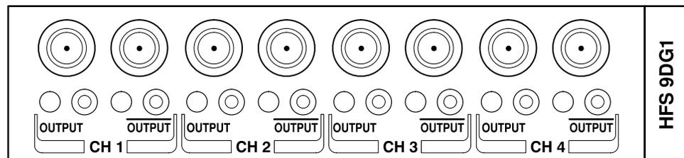
Figure 2-4: Channel Controls on an HFS 9DG1 Card
