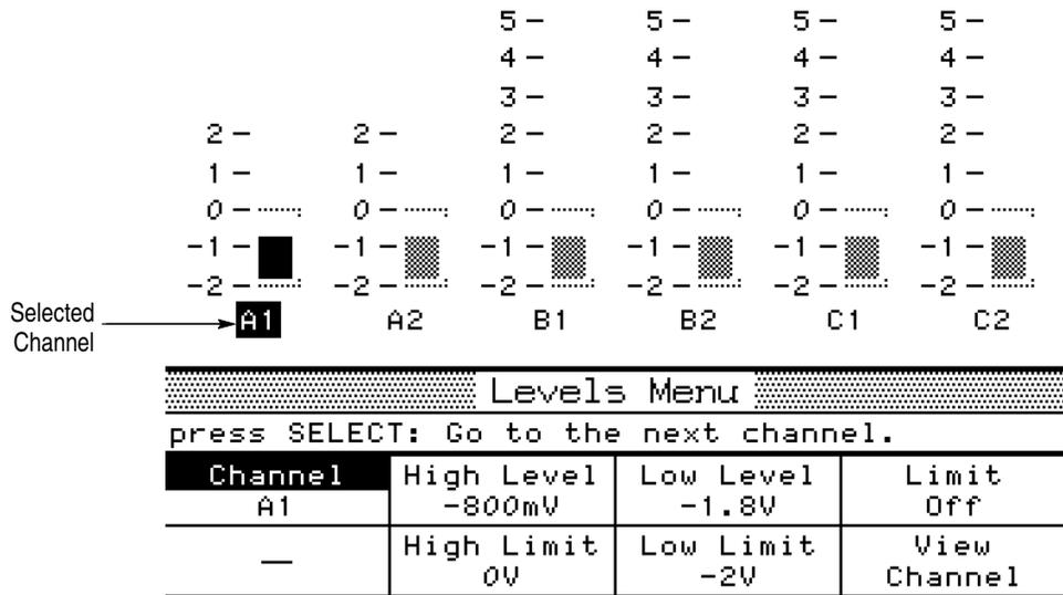
Figure 2-7: Levels Menu, Showing Channel Selection
