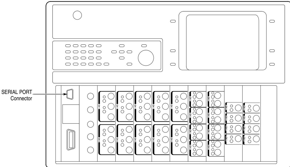
Figure 2-37: SERIAL PORT Connector Location
