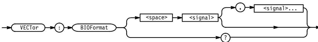
**Arguments** signal identifies the signal(s) to receive the data provided by subsequent BDATA commands.
