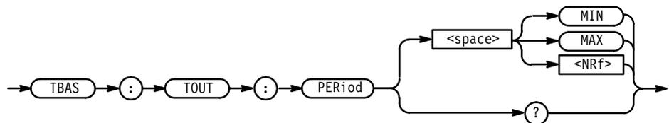
**Arguments** MIN sets the Trigger In level to 1.
