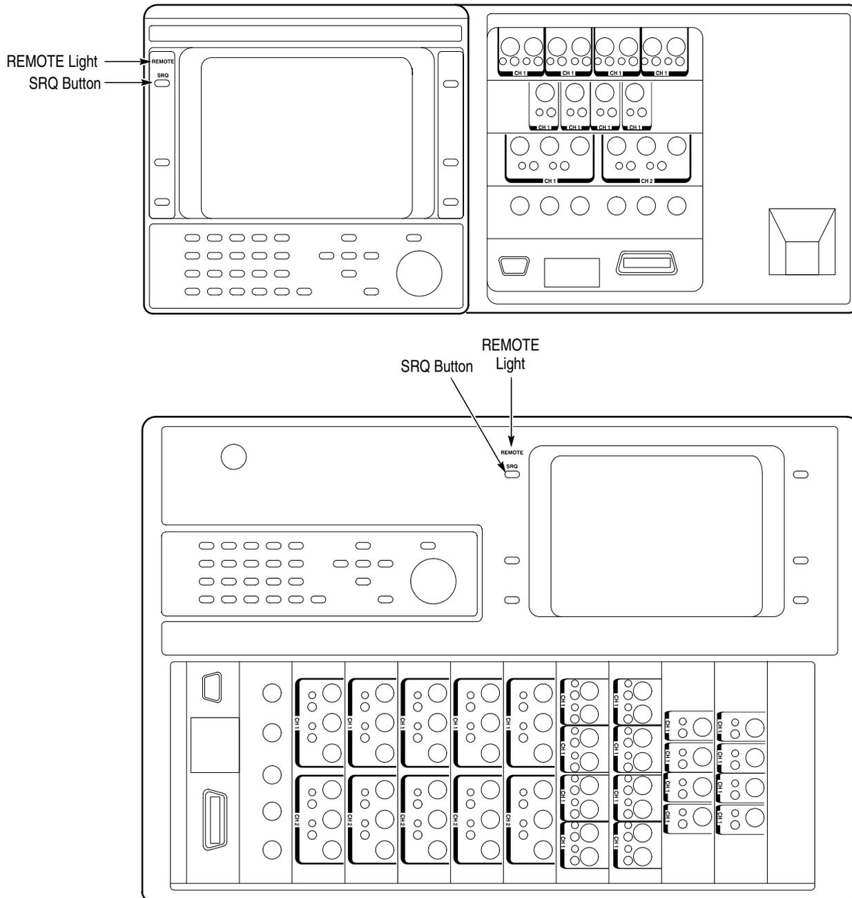
Figure 2-26: SRQ Button and REMOTE Light Locations
