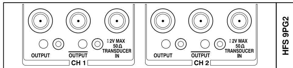
Figure 2-3: Channel Controls on an HFS 9PG2 Card
