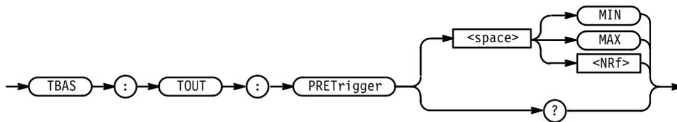
**Arguments** MIN sets the Trigger Out pretrigger to the minimum.
