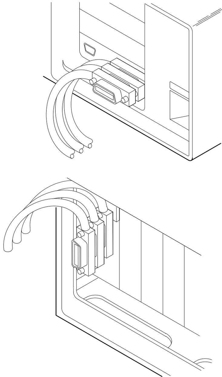
**Figure 3-2: How to Stack GPIB Connectors**
