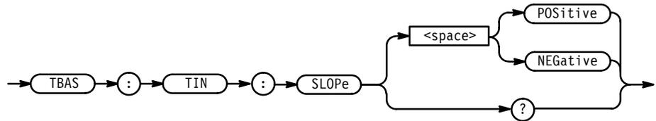
**Arguments** POSitive sets the Trigger In slope to positive edge triggering.
