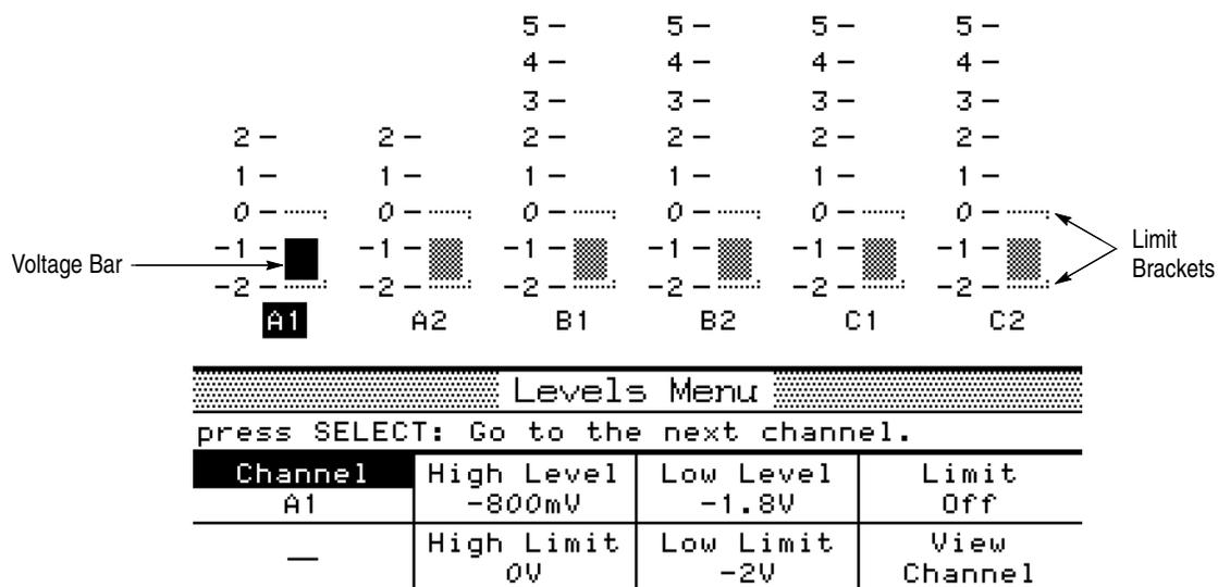
Figure 2-29: The Levels Menu and Associated Display
