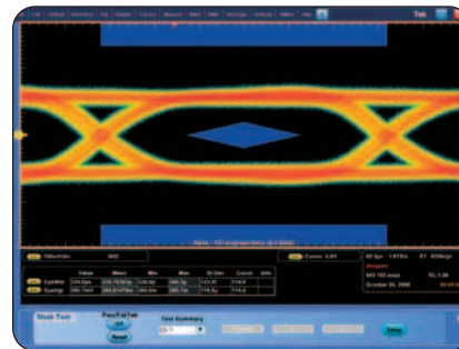
► Test eye diagram in equivalent time against the standard mask.
