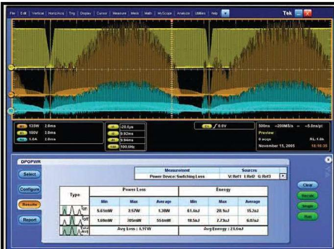
**Power Measurement and Analysis Software (Opt. PWR)** – Improve the efficiency of switching power supplies with increased power densities. Measure and analyze power dissipation in power supply switching devices and magnetic components, and generate detailed test reports in customizable formats.
