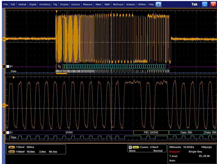
Triggering on a USB full-speed serial bus. A bus waveform provides decoded packet content including Start, Sync, PID, Address, End Point, CRC, Data values, and Stop.
