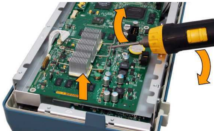
Figure 4-4: Disconnecting the Main board
