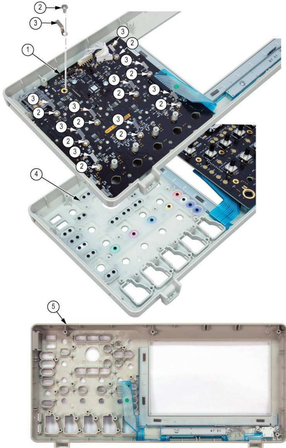
Figure 5-7: Exploded view: DPO3000 front panel board and front case
