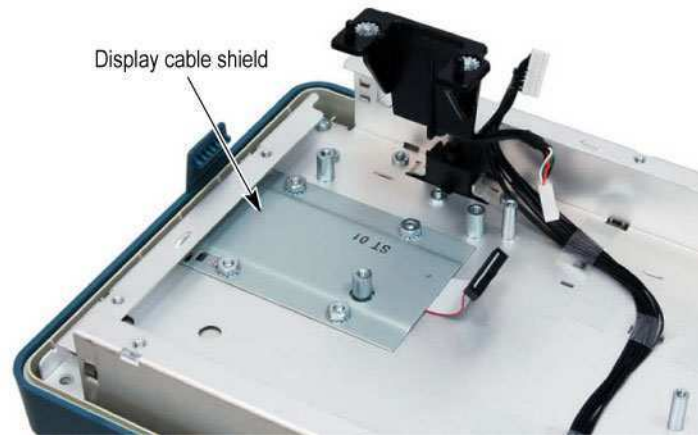
Figure 4-5: Display cable shield in place
