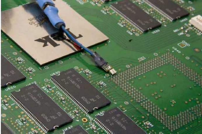
The low-cost solder tips available for the P7500 TriMode probes allow quick connection so moving the probe to various solder points is fast and easy.
