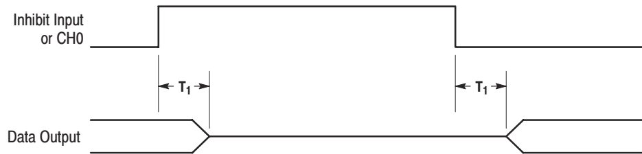
T 1 : The delay time from an external inhibit input or a CH0 signal until the corresponding data output goes to the high-impedance state, or the delay from the high-impedance state until high- or low-level data is available. Refer to Figure A-2 on page A-5 for more information.
