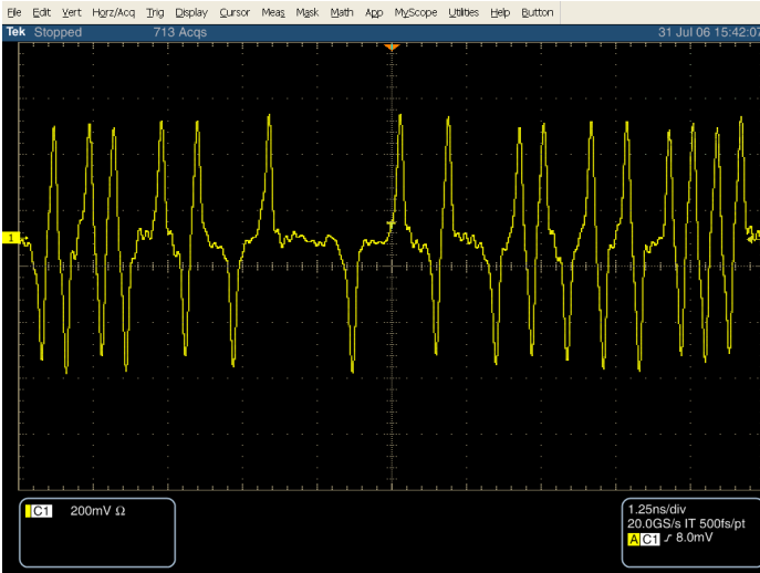
Figure 3: Hard disk read channel signal (5 Gb/s 2 points per cell); AWG7101 with 10 GS/s.
