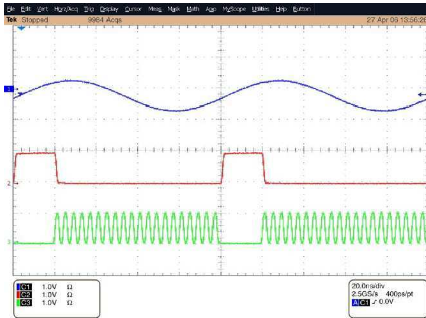
Figure 2-4: Output waveform from the Analog, Mkr1, and Mkr 2 connectors
