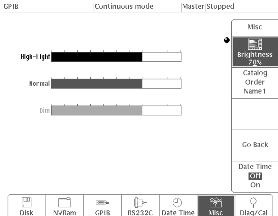
Figure 2-14: Setting the Display Brightness
