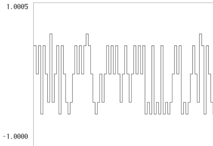
Figure C-16: \pi/4 DQPSK Q Axis Signal
