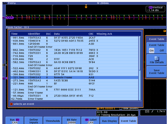
Event table for CAN bus with all captured packets time stamped and in a tabular view.
