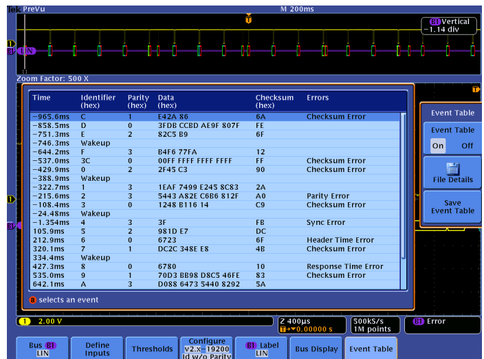
Event table for LIN bus with all captured packets time stamped and in a tabular view.
