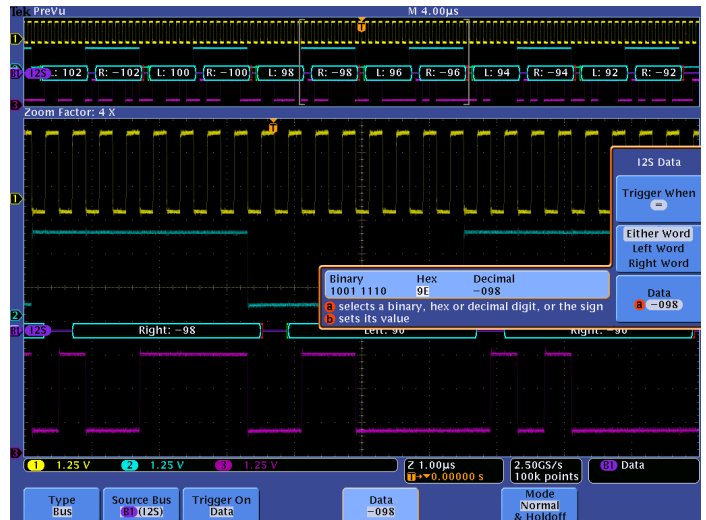
Triggering on a specific data value on the I 2 S bus.
